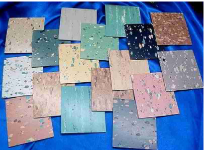
Asbestos Floor Tiles
